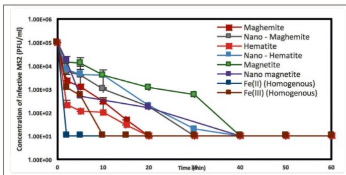
Fig. 1. Inactivation of MS2 virus by homogenous and heterogenous photo-Fenton (Solar irradiance 900W/m<sup>2</sup>. Concentration of iron, iron oxides, H<sub>2</sub>O<sub>2</sub> = 1mg/L)
